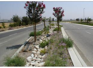
A median with a small river stone drainage bed and drought-tolerant plants
